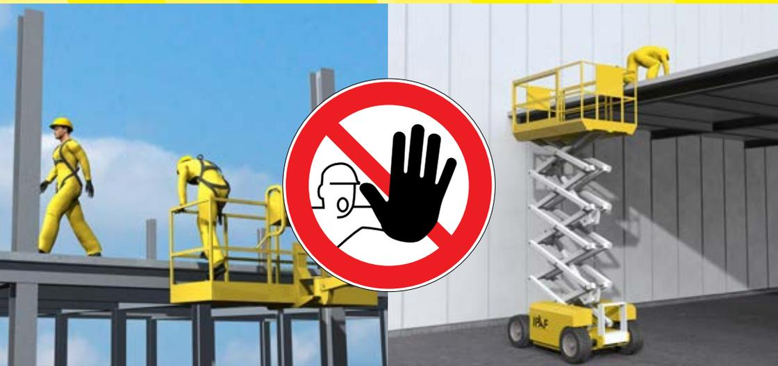
**Mobile elevating work platforms (MEWPs) are specifically designed to lift people to a position where they can work at height safely within the platform.**
